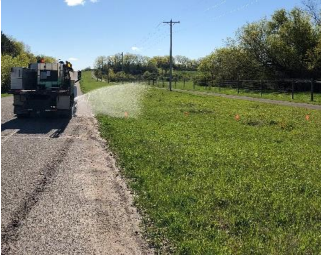
Figure 1: Boomless sprayer applying herbicide to a ROW infested with invasive species
